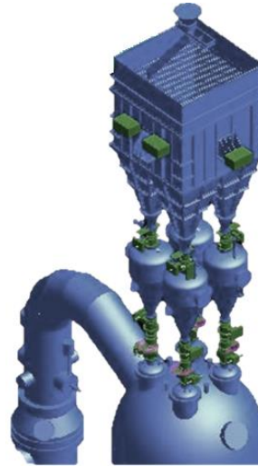
Iron ore charging system
