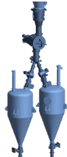
DRI discharging system
